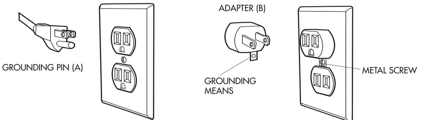
USE OF AN ADAPTER IS NOT ALLOWED IN CANADA. IF A GROUNDING TYPE RECEPTACLE IS NOT AVAILABLE, DO NOT USE THIS APPLIANCE UNTIL THE PROPER OUTLET IS INSTALLED BY A QUALIFIED ELECTRICIAN.
